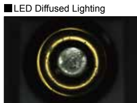
It is difficult to evenly illuminate the whole solder.
