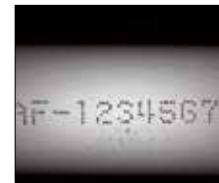
Inspecting dot-marked characters on pipe Light used: LSP-41RD
