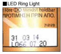
Illuminated light converges in the center, making stable inspection difficult.
